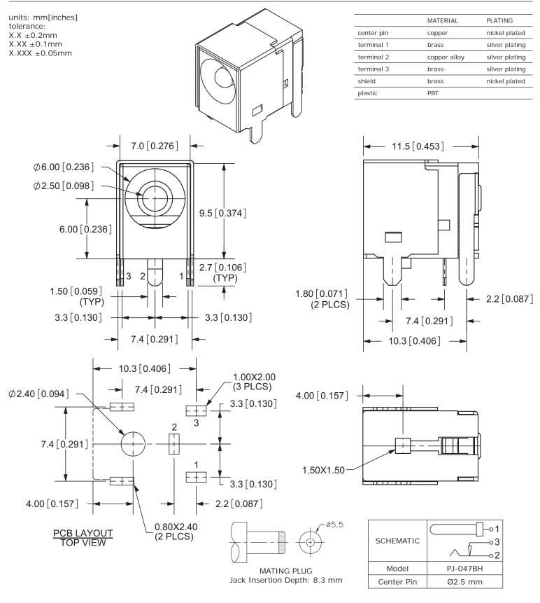
1. All specifications measured at 10~35°C, humidity at 45~85%, under standard atmospheric pressure, unless otherwise noted. Note: ..... ..... CUI Inc | MODEL: PJ-047BH | DESCRIPTION: DC POWER JACK
